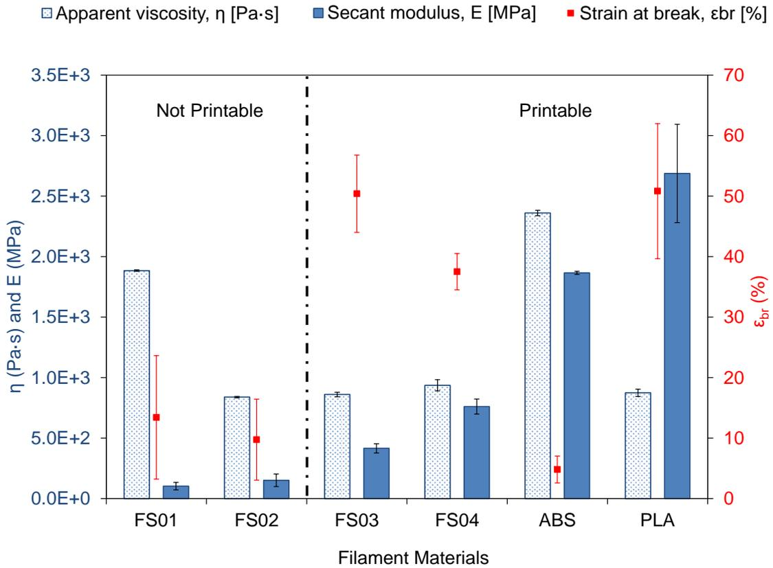
Figure 2. Viscosity and mechanical properties of printable and not printable filaments.
