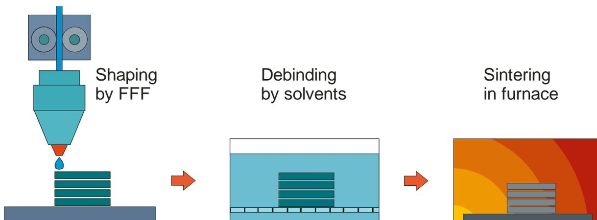
Figure 1. Schematic representation of the SDS process
