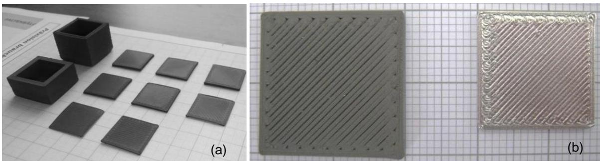
Figure 3. (a) Printed parts produced with feedstock materials FS03 and FS04; (b) greenpart shaped by FFF and final part after debinding and sintering.
