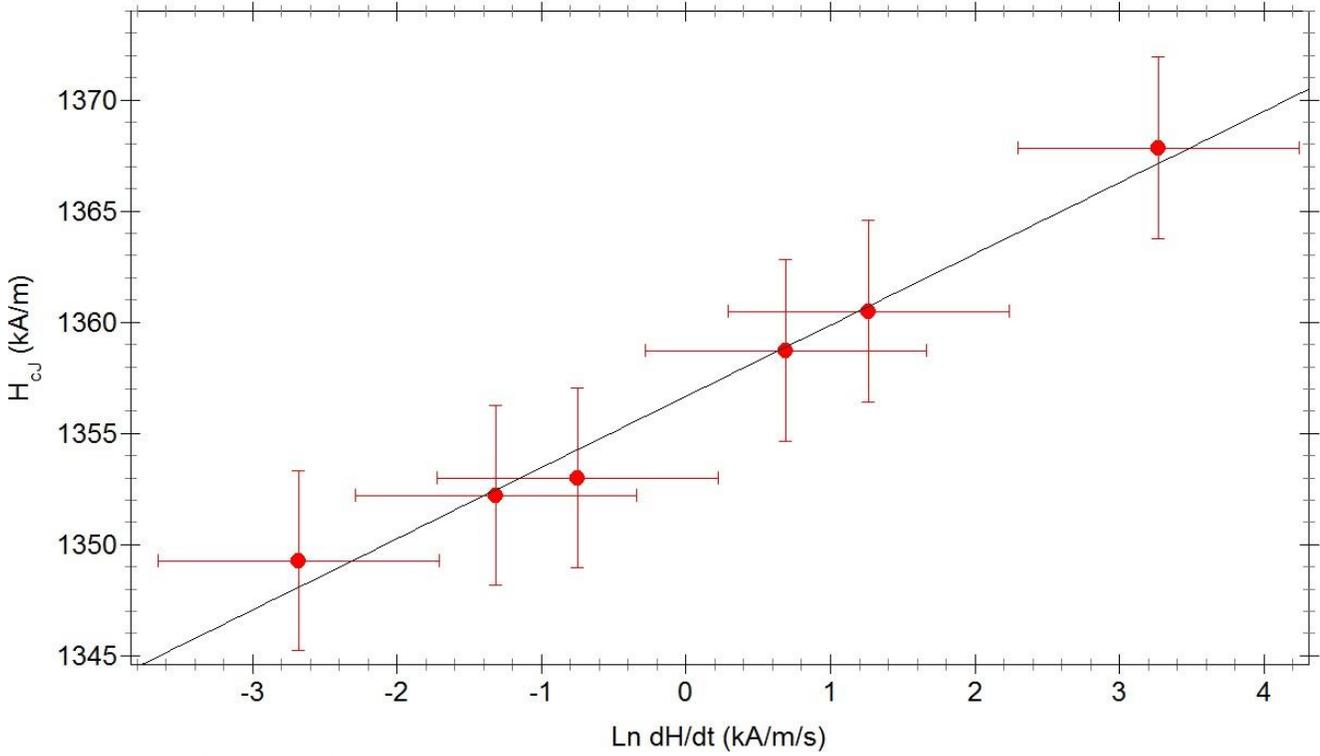
Fig.4. The plot of  $\ln(dH/dt)$  against measured coercivity displaying the expected linear behaviour
