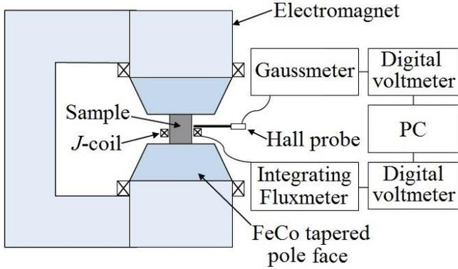
Fig. 2. A schematic of the electromagnet set-up taken from [11].
