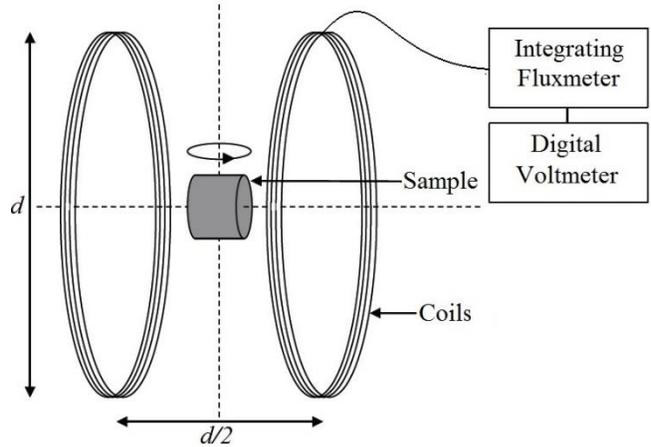
Fig. 3. Schematic of the Helmholtz coil used for the determination of  $m_k$ .  $d/2$  is equal to 130 mm for this set up.
