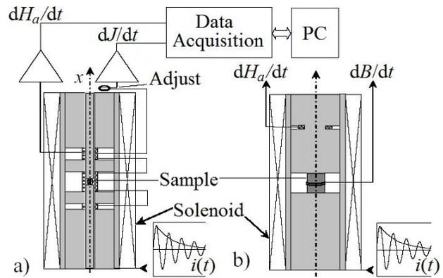
Fig. 1. Schematic of a PFM [5] where in a) the pick-up coils couple to the flux at the ends of the sample and in b) the pick-up coils couple to the flux at the mid-plane of the sample.
