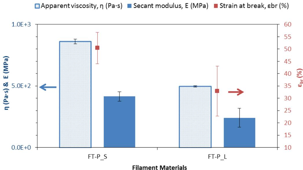
FIGURE 3. Apparent viscosity ( $\eta$ ), secant modulus ( $E$ ) and elongation at break ( $\epsilon_{br}$ ) for filaments with different particle sizes.
