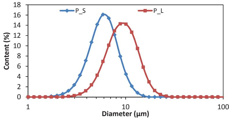
**FIGURE 1.** Particle size distributions of 316L stainless steel powders (P\_S, small and P\_L, large) measured by laser scattering.
