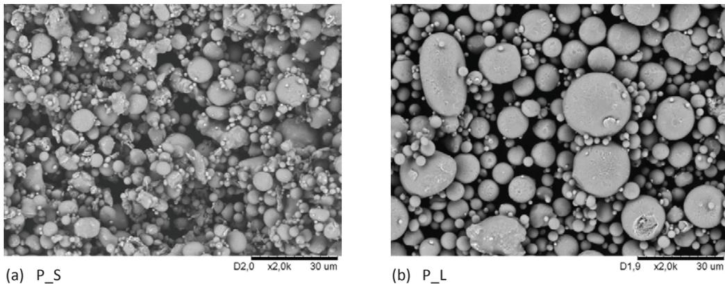
**FIGURE 2.** Scanning electron microscopy images of 316L powder (a) P\_S, small and (b) P\_L, larger particles.
