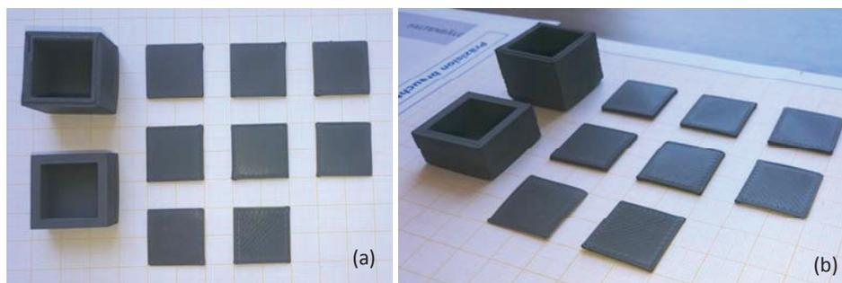
**FIGURE 4.** Parts produced by FFF using filaments with FT-P\_S feedstock material (a) top view and (b) side view.
