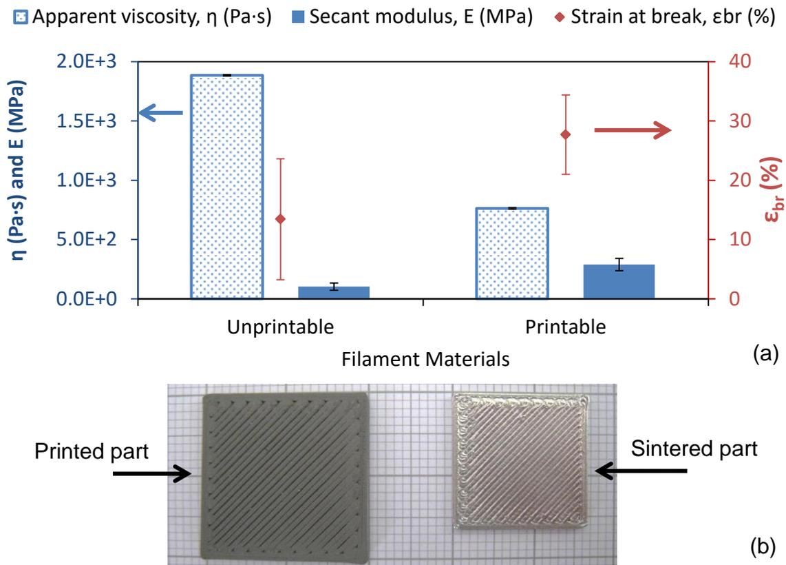
Figure 1: (a) Material properties of printable and unprintable materials;
