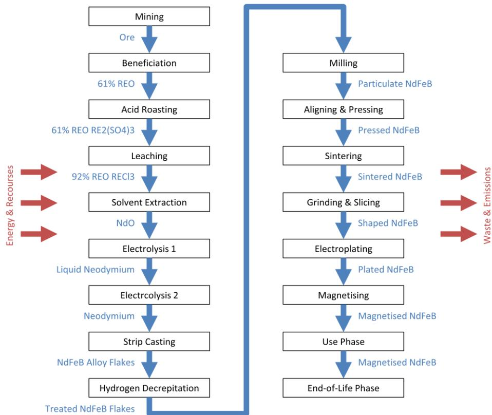
Figure 1 - State-of-the-art process chain.
